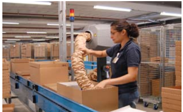
In line packaging using a Chevron machine.
